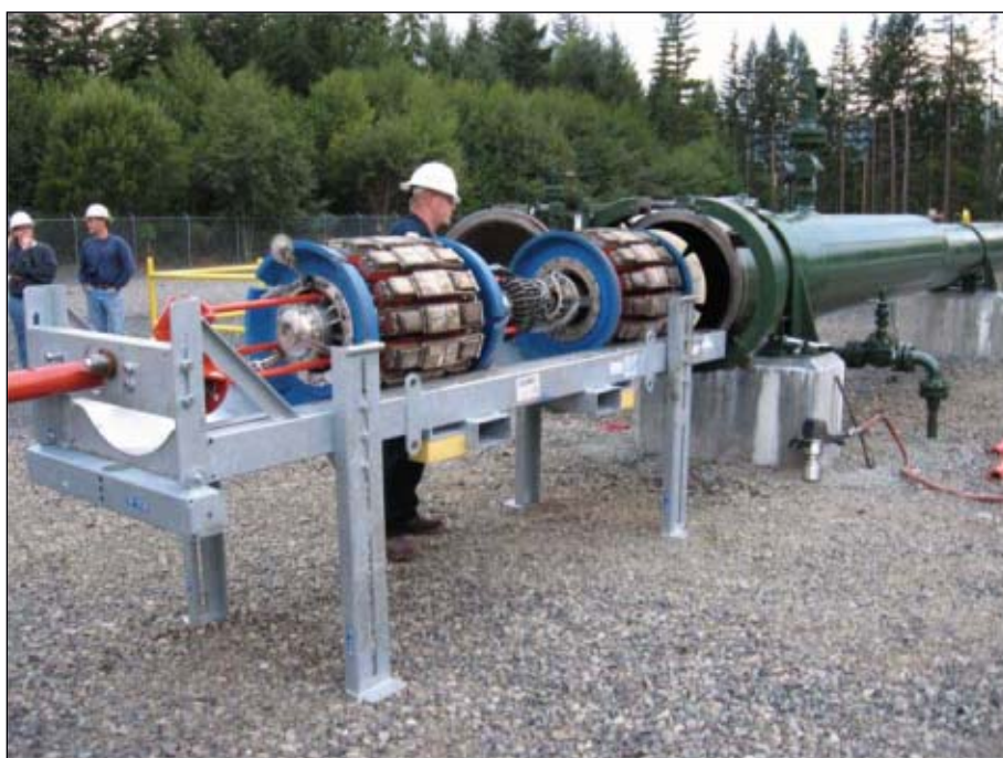
A technician prepares a 24-26-in. multidiameter EMAT in-line inspection tool for launch. Achieving full high-resolution coverage around the circumference of the pipeline requires equipping two measurement units with a sufficient number of sensors (Fig. 1).
